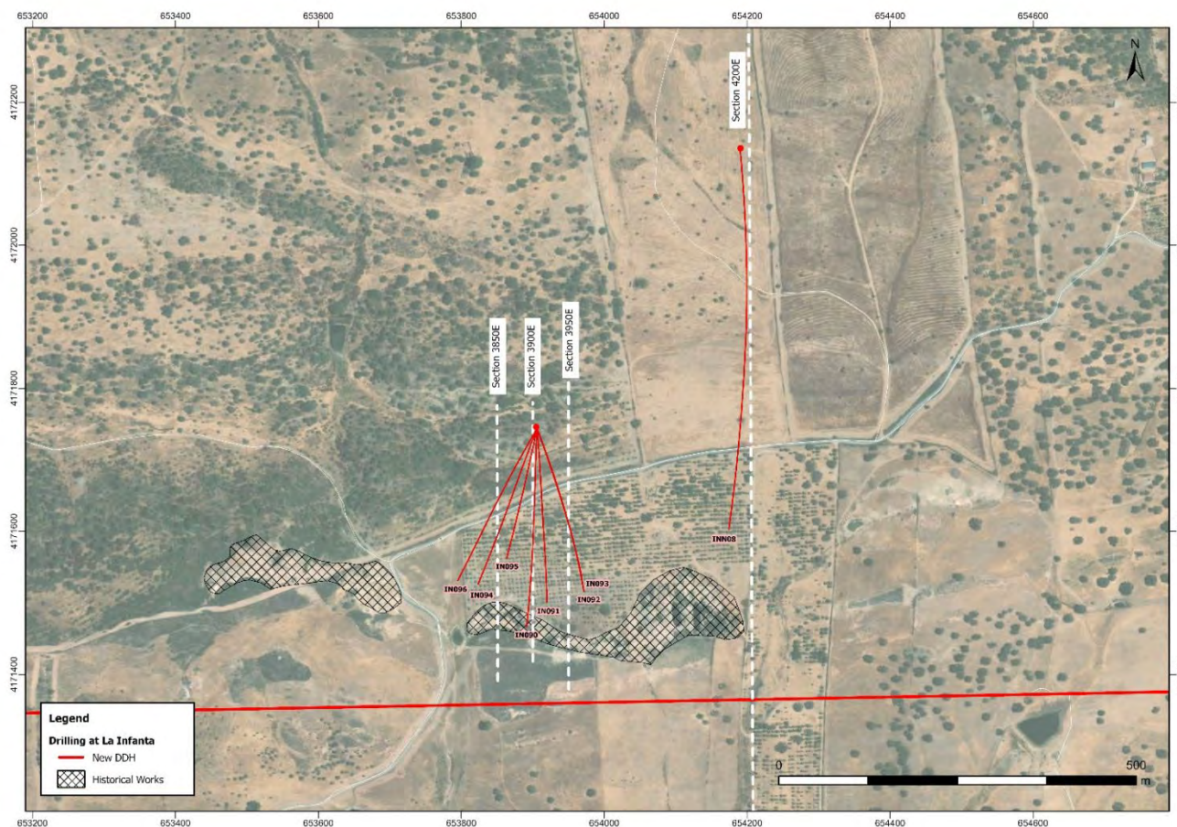
Figure 2. Plan view map showing drill hole traces and section lines of La Infanta drilling. Hole traces in this release are colored red. IBW tenement boundary shown as east-west red lines.
