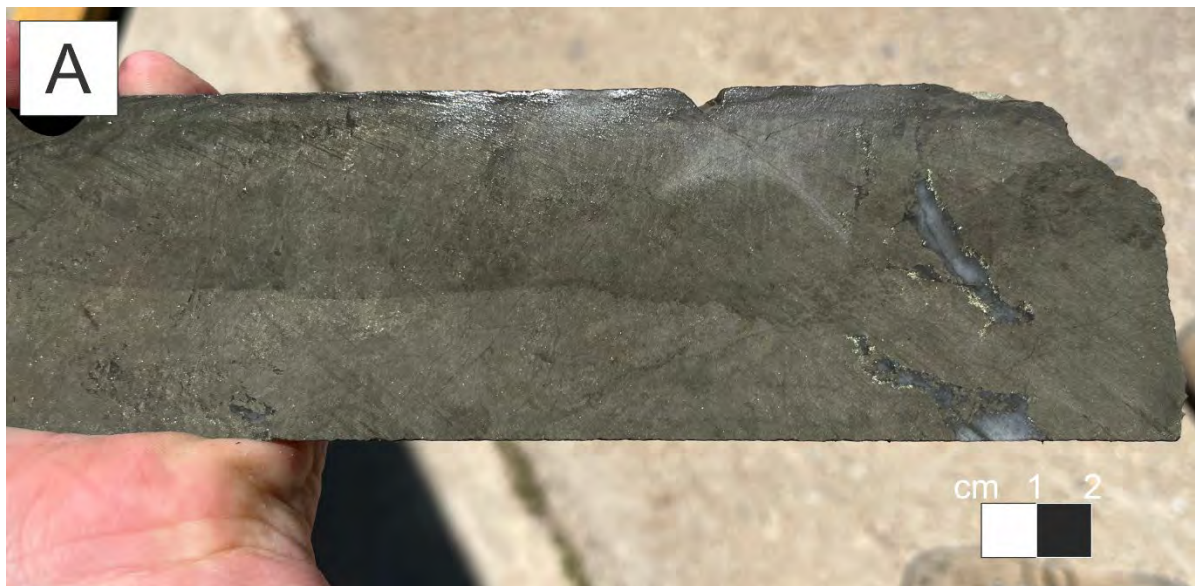
Figure 5. Photos of El Cura drillcore as described in this release: A: EC051; Fine grained massive sulphide. Visible chalcopyrite along fracture planes and irregular veinlet.
