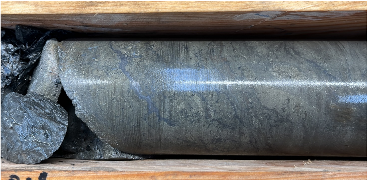
Figure 5. Core photos of EC018 polymetallic massive sulfide with galena vein.
