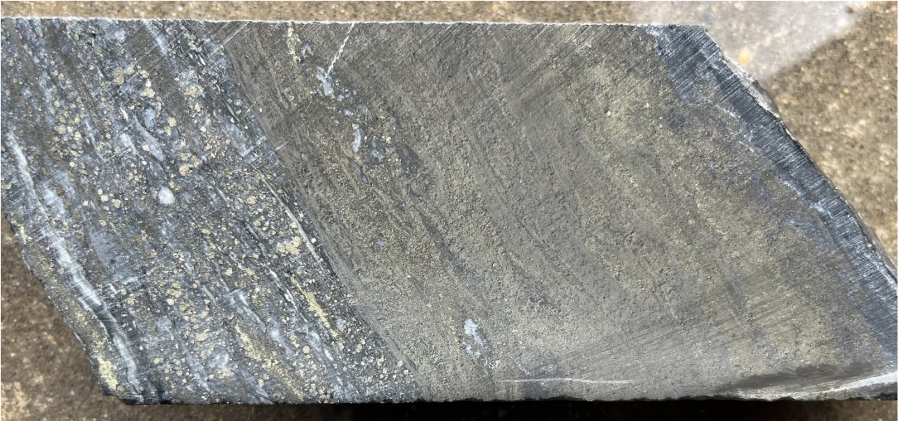
Figure 6. Core photos of EC019 polymetallic massive sulfide with galena vein.
